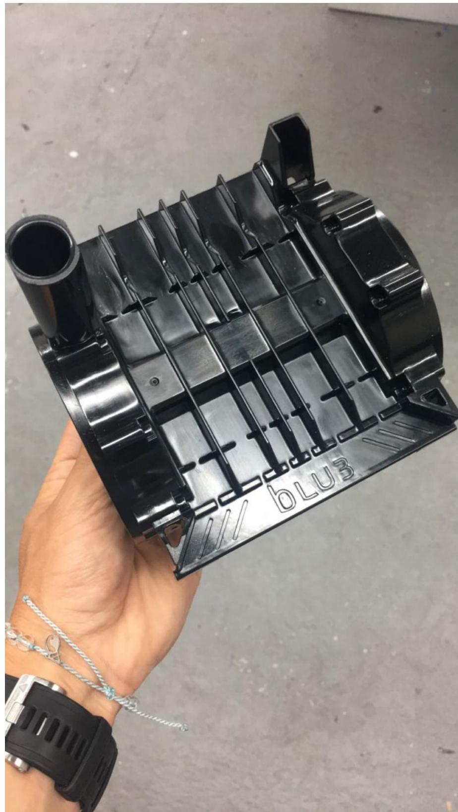
*Injection Molded Pump Body – a very complex part!*
