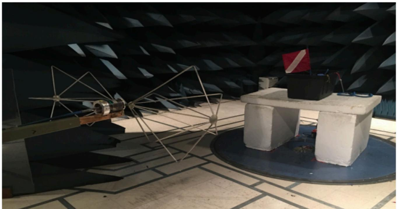
Two Nemo prototypes were taken to a compliance testing lab this week where the radiated electromagnetic emissions were evaluated. This test was a form of preliminary testing to get an idea of where we stand before proceeding into the full formal testing, which will take place over the course of 4-5 days in the beginning of April. The testing is a requirement for obtaining FCC and CE certifications.
