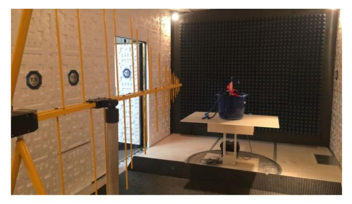
Successful completion of EMC testing is a requirement for communications certifications around the world, such as FCC in the United States and C-tick in Australia. Most certifications require only the emissions testing portion of the EMC test. Since we plan to
